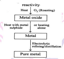
Metal sulphide like HgS reacts with  $O_2$  on heating to from mercuric oxide, HgO and sulphur dioxide Mercuric oxide on further heating gives Hg which can be refined by distillation.
